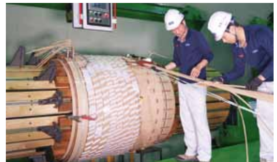
Interleaved Winding
