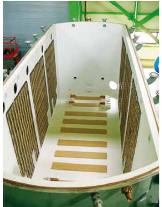
· TANK & MAGNETIC SHIELD
