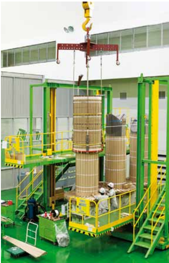
· CORE AND COIL ASSEMBLY
